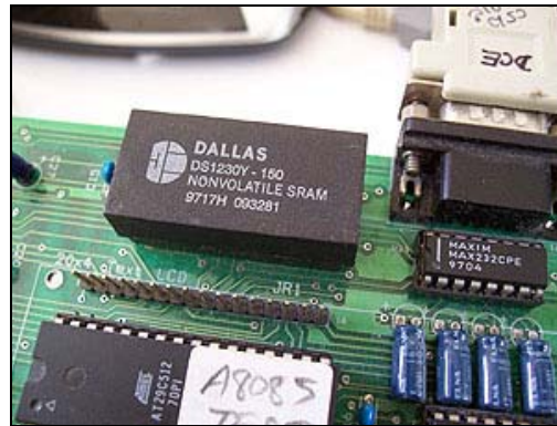
Figure 13: Using DALLAS DS1230, 32kB NVRAM for user program running.
