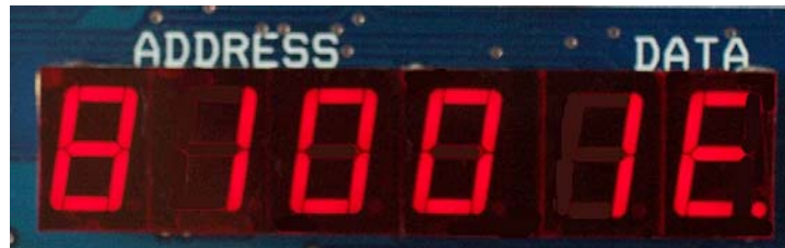
Figure 3: The LED shows memory location 8100 and its content, 1E.
